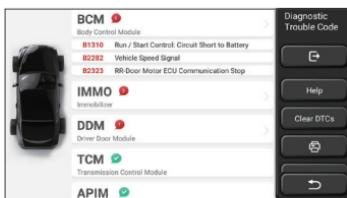
The system with DTC will be displayed on the screen in red font, and the specific number of DTC will be shown. A DTC-free system will be displayed as "OK".
