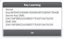
c. Place the new key into the programmer key slot and touch **OK**.
