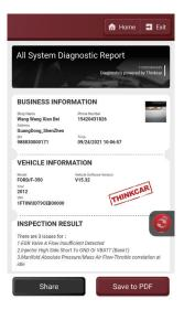
B. System Scan: what systems the vehicle are equipped with are automatically scanned.
