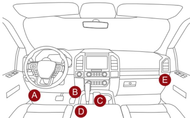
Usually, the OBD port is located under the dashboard, above the pedal on the driver's side. The five locations shown in the picture are common OBDII port locations.
